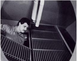
The TB droplet separator is a stable and solid packing unit. The unit consists of individual plastic elements linked by a central plastic rod.
