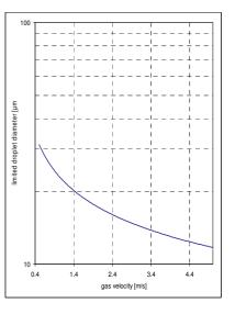
\* The limited droplet diameter corresponds to the smallest diameter of droplet (12  $\mu$ m) removed from the gas stream at a velocity of 3 to 4.5 m/s at a pressure drop of 5 to 14 mm water-column.
