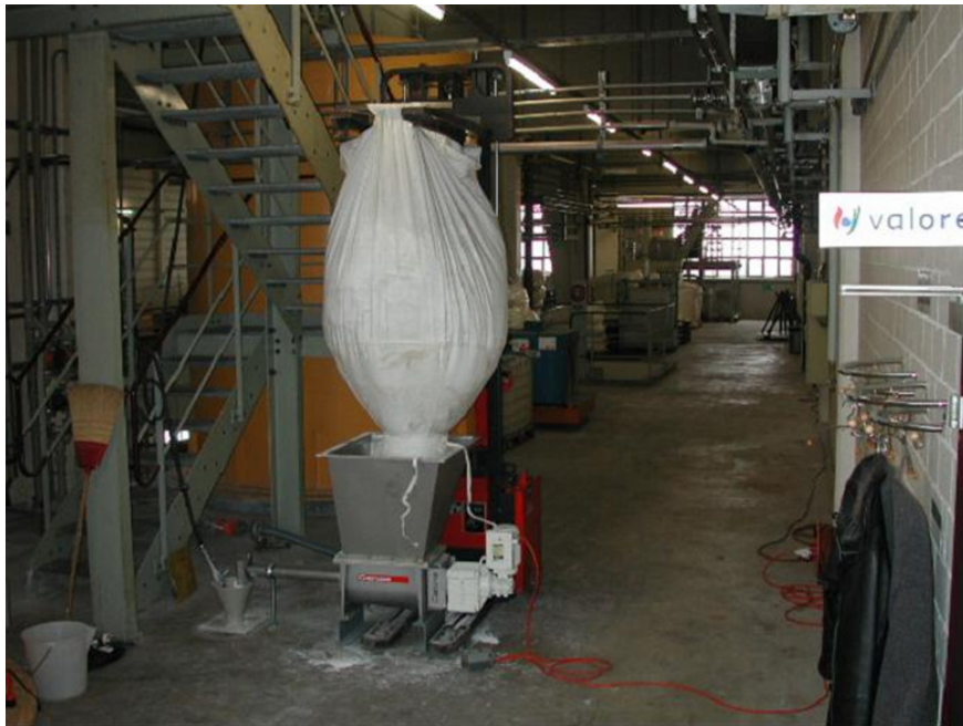
Figure 2: A big bag of sodium carbonate ashes is fed at various rates to neutralize scrubber liquors
