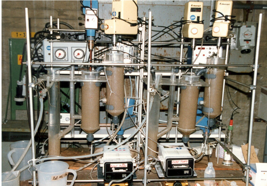
Figure 1: Two activated sludge treatment trains consisting of 2 serial treatment tanks followed by a sedimentation tank. The plant on the left was aerated while the plant on the right was fed with nitrate.
